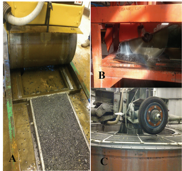
Fig. 2: CRS test preparation, A- compacting the asphalt slabs, B- sawing the asphalt slabs, C- fitting and gluing of the asphalt slabs on the circular track of the CRS
